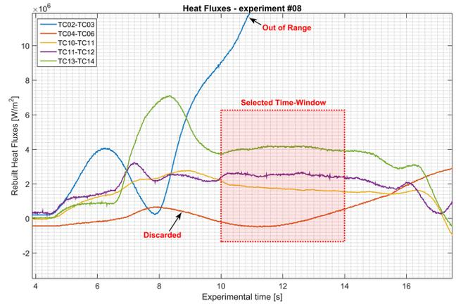
**Figure 19: Heat-flux rebuilding for experiment #08**
