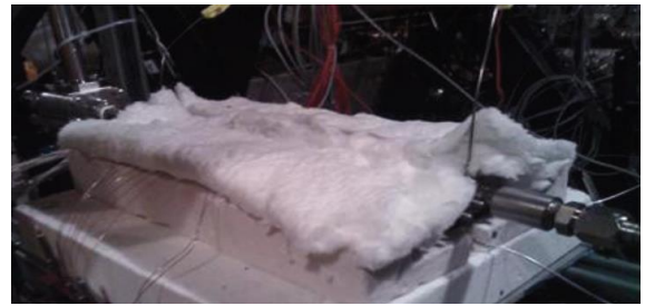
Figure 9 - Insulated MTP on test stand during testing
