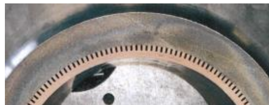
Figure 31 - Brazed 'dummy' chamber, cylindrical part section.
