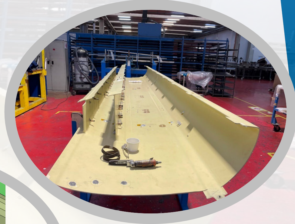
HIGHLY INTEGRATED CFRP STRUCTURE
