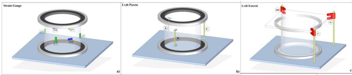
**Figure 13.** Strain gauges and LVDT locations
