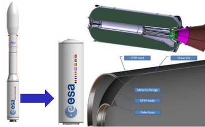
**Figure 1:** SRM case architecture.
