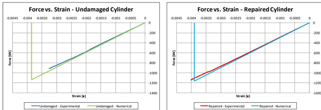
**Figure 17.** Comparison between numerical and experimental results
