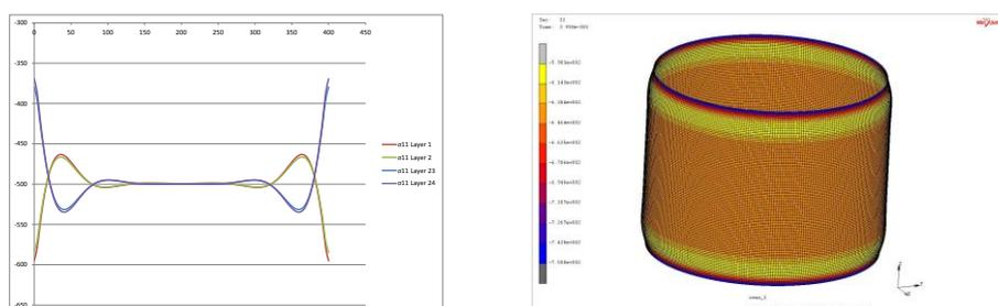
**Figure 10.**  $\sigma_{11}$  in inner and outer 0° ply and failure elements at 1140 kN
