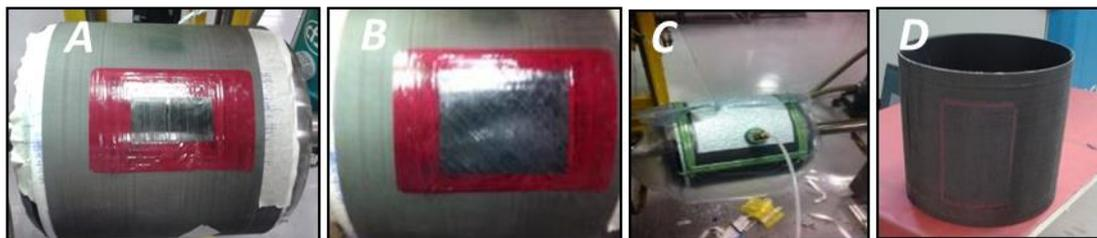
**Figure 9.** Hand lay-up of the repairing patch, vacuum bag and repaired scaled cylinder Skirt
