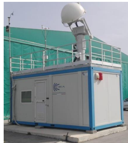
GCS and telemetry antenna
