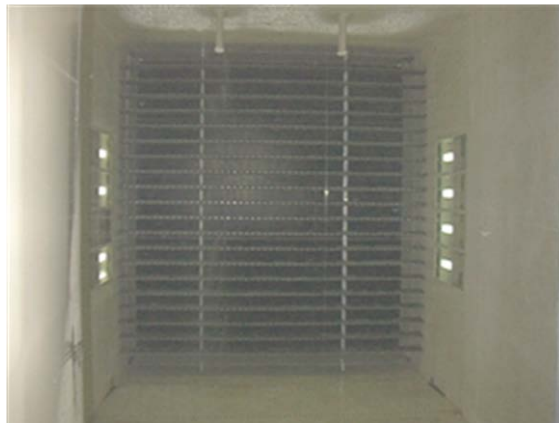
Figure 2: CIRA-IWT Spray bar view from the test section.
