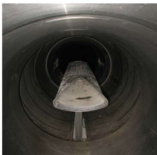
Fig. 39. Scramjet module installation in the facility.
