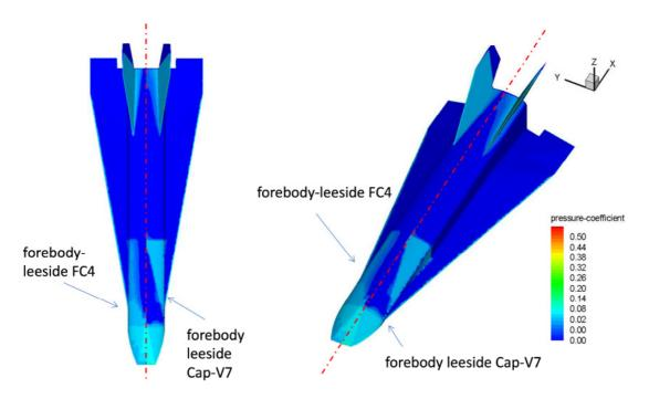
Figure 9: Pressure distribution comparison between CIRA-C4 and CIRA-FC4.
