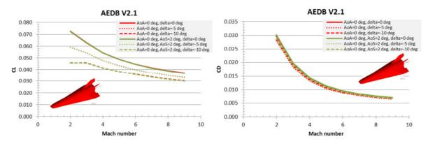
Figure 17: C<sub>L</sub> and C<sub>D</sub> vs. Mach number with and without sideslip angle and aileron deflection effects.
