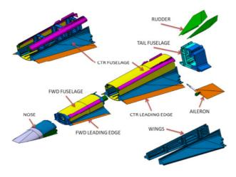
Figure 14: EFTV main components
