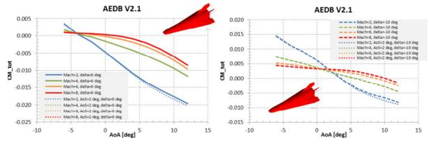
Figure 21: C<sub>m</sub> versus AoA at different Mach numbers and with and without sideslip angle effects.
