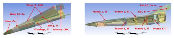
Figure 25: Main structural components of the analysed EFTV
