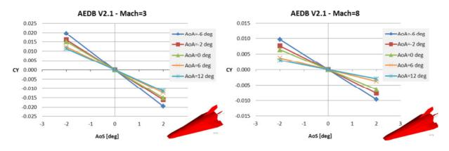
Figure 22: C<sub>Y</sub> versus AoS at different AoA at M<sub>∞</sub>=3 and 8.
