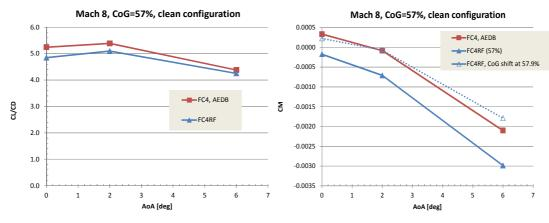
Figure 12: Aerodynamic performance comparison at M=8 between CIRA-FC4 and CIRA-FC4RF.
