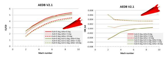
Figure 18: L/D and C<sub>m</sub> vs. Mach number with and without sideslip angle and aileron deflection effects.
