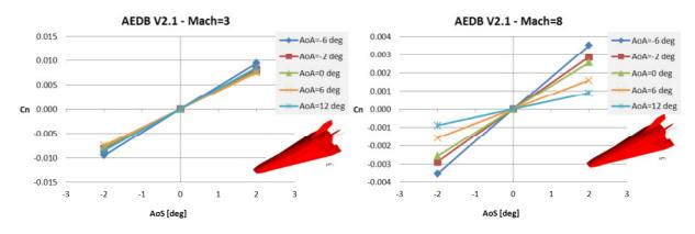
Figure 24: C<sub>n</sub> versus AoS at different AoA at M<sub>∞</sub>=3 and 8.
