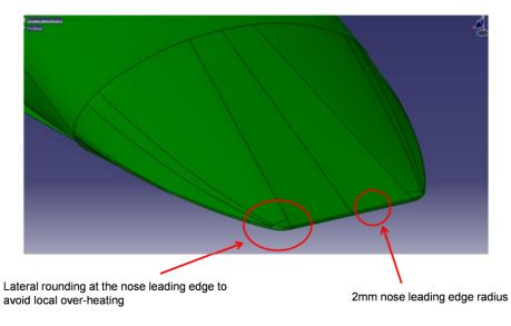
Figure 11: CIRA-FC4RF details of the forebody leading edge.
