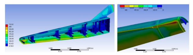
Figure 27: Temperature distribution on the titanium structure at the peak heating condition for titanium components
