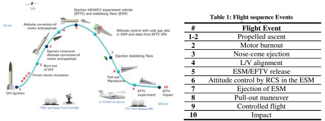
Figure 2: Flight sequence profile
