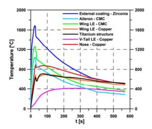
Figure 26: Maximum temperature along the flight profile on the main vehicle components
