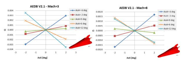
The sideslip derivative of the rolling moment coefficient  $C_1$  is provided in Figure 23 at five angles of attack, namely -6, -2, 0, 6, and 12 deg. As one can see, dihedral effect stability is predicted at all Mach numbers for AoA  $\ge 0$  deg.
