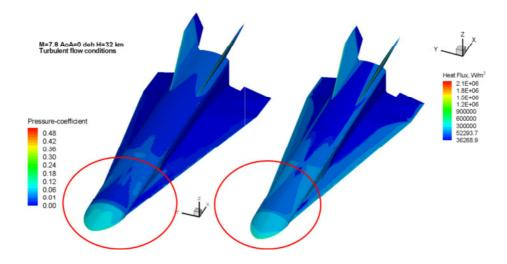
Figure 7: Pressure and heat flux surface distributions for the DLR-Cap\_7 aeroshape.
