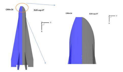
Figure 5: EFTV forebody. Comparison between DLR-Cap\_V7 and CIRA-C4 aeroshapes.
