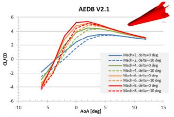
Figure 19: L/D vs. AoA at M=2, 4, 6, 8 and for 0 deg and -10 deg aileron deflections.
