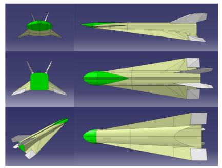
Figure 4: EFTV Cap\_V7 aeroshape by DLR.
