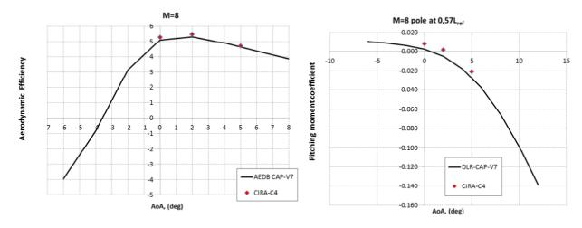
Figure 6: Comparison between DLR-Cap\_7 and CIRA-C4 in terms of L/D and Cm.
