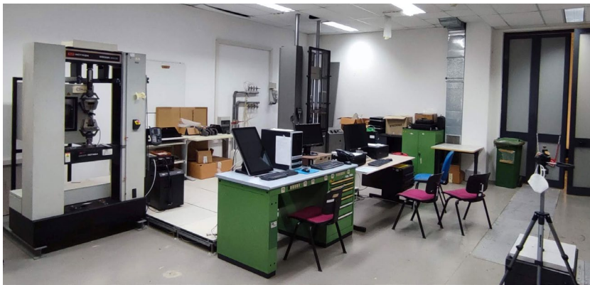
Destructive material testing: Static Electromechanical Material Testing up to 100kN, Dynamic Hydraulic Material Testing up to 250kN, High Deformation Rate Material Testing up to 20 m/s
