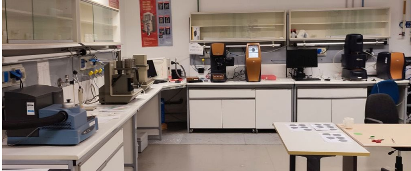
Calorimetric and rheological analysis: Modulated Scanning Differential Calorimetry, Thermomechanical Analysis, Dynamic Mechanical Analysis, Thermogravimetry, Rotational Rheometer
