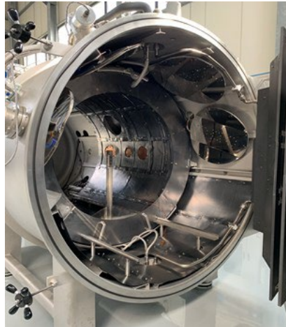
Internal view of the facility with the cryo-panels visible.
